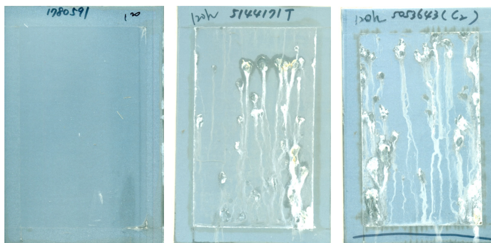
Fig.10. Salt spray test with 120 hours of each sample. (a) Cr-free A; (b) Cr-free B; (c) Cr
